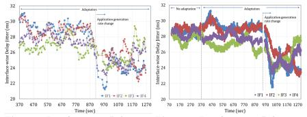
Fig. 9: Interface-wise Delay jit-Fig. 10: Interface-wise Delay jitter performance using Model ter performance in Experiment (Equation 9). (Traffic: RTP, N = 4) (Equation 1). (Traffic: RTP, N = 4)
