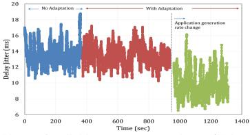
Fig. 13: Overall delay jitter variation with time (Without adaptations and adaptation in the same run). (Traffic: RTP, N = 4)
