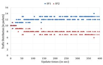
**Fig. 4**: Convergence of traffic distribution (in packets) with time on applying the adaptation algorithm at the sender.
