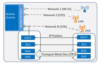
**Fig. 1**: A Multi-Access System with Wi-Fi and LTE connections, and emphasizing the user plane protocol stack interaction for the LTE connection in a multi-access system.
