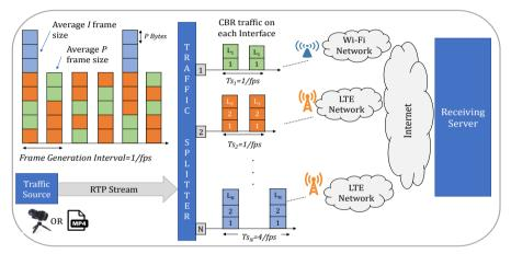
Fig. 2: A Multi-Access System and video traffic splitting across multiple interfaces.
