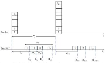
Fig. 3: SILA Model with delays and timestamps for an interface.
